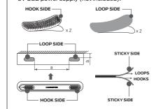
a: 6.15 inch between 2 velcro b: ≥0.7 inch from velcro to the wall 2. Install with base support
